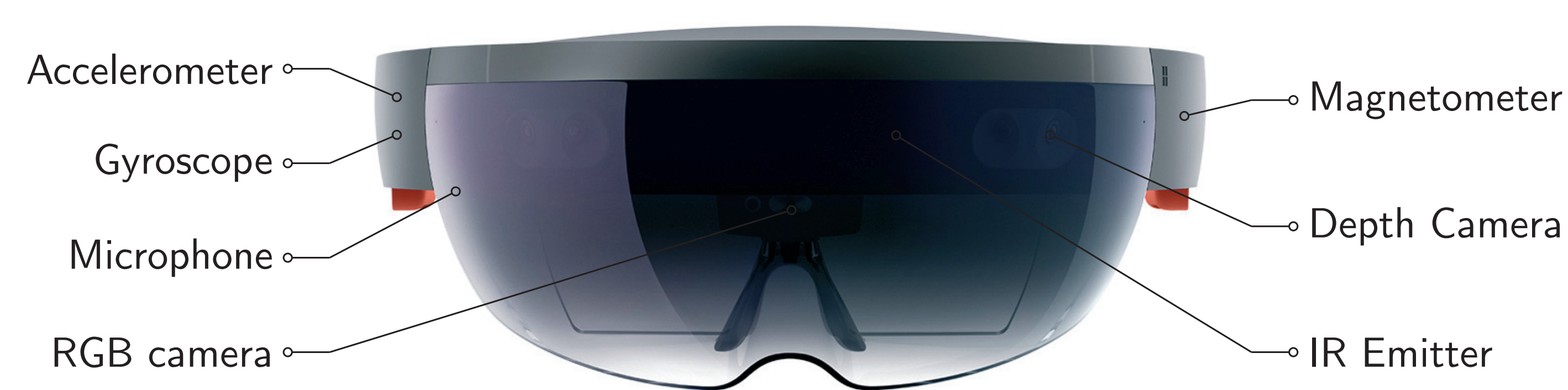
Figure 1. Sensors in the HoloLens
