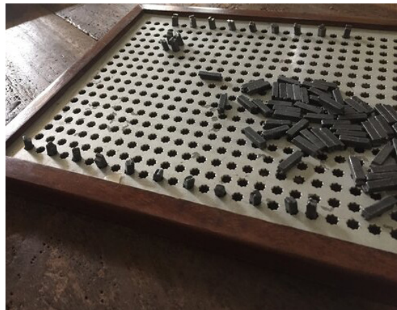
A Taylor frame can be used to create graphs: the type is used to mark the axes and points.
