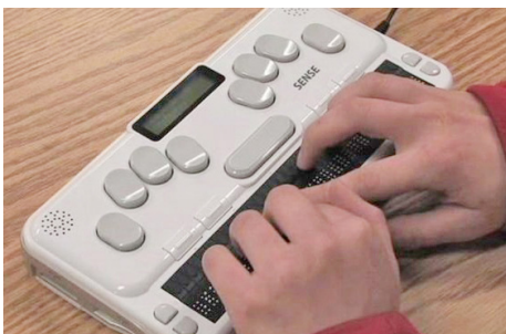
A braille notetaker. The keys at the top are used to input text. The user's hands are on the refreshable braille display.
