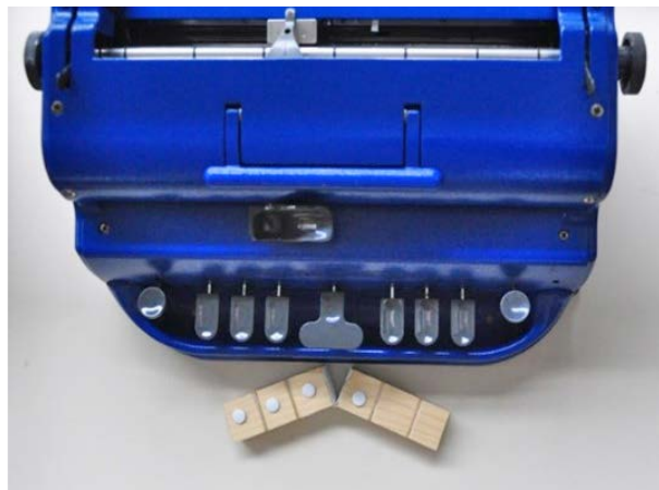
This braille cell block opens up to show the relationship between the braille dots and the keys on the braille. The pegs are removable to depict different braille signs.
