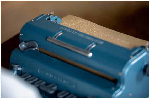
A Perkins braille is a typewriter that embosses braille signs into heavy paper.
